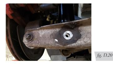
6. Attach the shock to the lower control arm. Torque at ride height 50Nm + 90 degrees (37 lb.-ft. + 90 degrees) (Fig. D.21).
