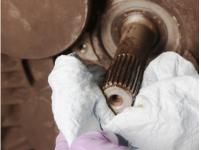
15. After cleaning the mounting boss, install the new slave cylinder and tighten the fixing screws to 16 N.m (12 Lb.Ft)
