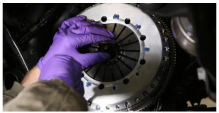
23. Tighten each of the pressure plate screws by another full turn in a criss cross fashion. Repeat until there is no gap between the pressure plate and the flywheel.
