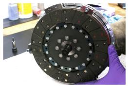
19. Install the clutch pack and both discs onto the flywheel by aligning the alignment tool to the center of the crankshaft.
