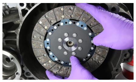
14. Remove the excess grease from the disc and input shaft, leaving only a VERY thin layer on the splined section of the shaft. Any excess grease will spin off the input shaft and contaminate the friction material; causing slipping, chatter, glazing, and other engagement issues. Contaminated friction material is not covered under warranty.
