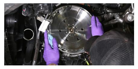
8. Install the crank bolts finger-tight only. Do not tighten them yet.
