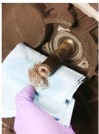
11. Use a clean rag to apply new grease to the input shaft splines.
