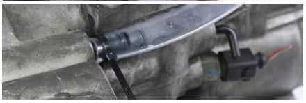
3a. Pour brake fluid into the funnel that is connected to the hydraulic bearing.
