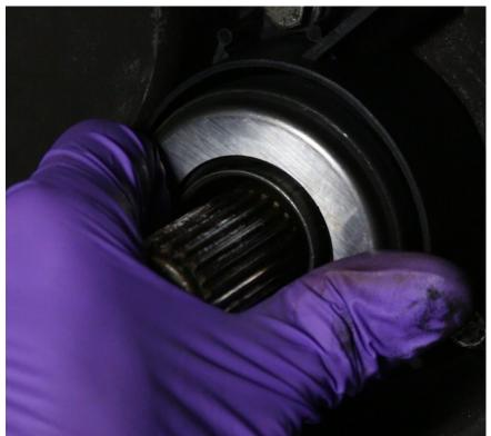
5a. Cycle the bearing until the bubbles are small and consistent. This step is to remove the majority of the air in the line. Any remaining air will be purged when final bleeding is performed in the vehicle.
