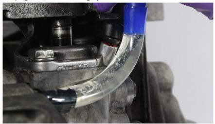
Tip: When later installing transmission the bearing will be compressed and fluid will be pushed out of the slave cylinder. As a suggestion you may want to zip tie a glove to the spout of the slave cylinder to catch the excess
