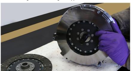
18. Place the bottom disc onto the alignment tool (hold the bottom disc and alignment tool, do not touch the friction surfaces).
