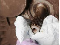
After cleaning the mounting boss, install the new slave cylinder and tighten the fixing screws to 16 N.m (12 Lb.Ft)
