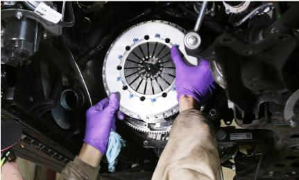
20. Start the screws into the pressure plate and finger-tighten them. Do not fully tighten the screws yet.
