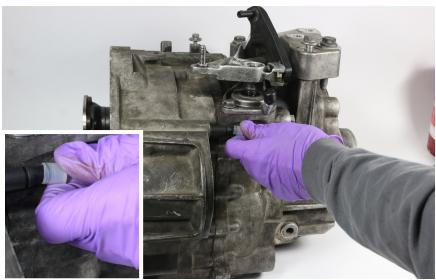
2a. Secure the funnel to the hydraulic bearing feed line.
