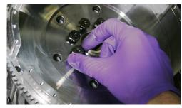
9. Prevent the flywheel from rotating with a flywheel locking mechanism and torque the crank bolts to 95 N.m (70 Lb.Ft) in a crisscross pattern.
