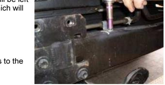
8. Take off the 2 bolts holding the cooler lines to the crossmember.
