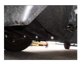
4. Once the skid plate is removed you will have access to 2 bolts on each side that hold another bumper support piece to the frame. Remove these 2 bolts from each side.
