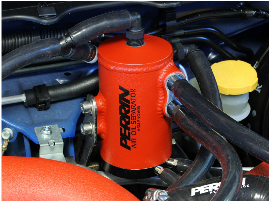
Above shows completed installation of AOS on an car with a PERRIN FMIC installed.
