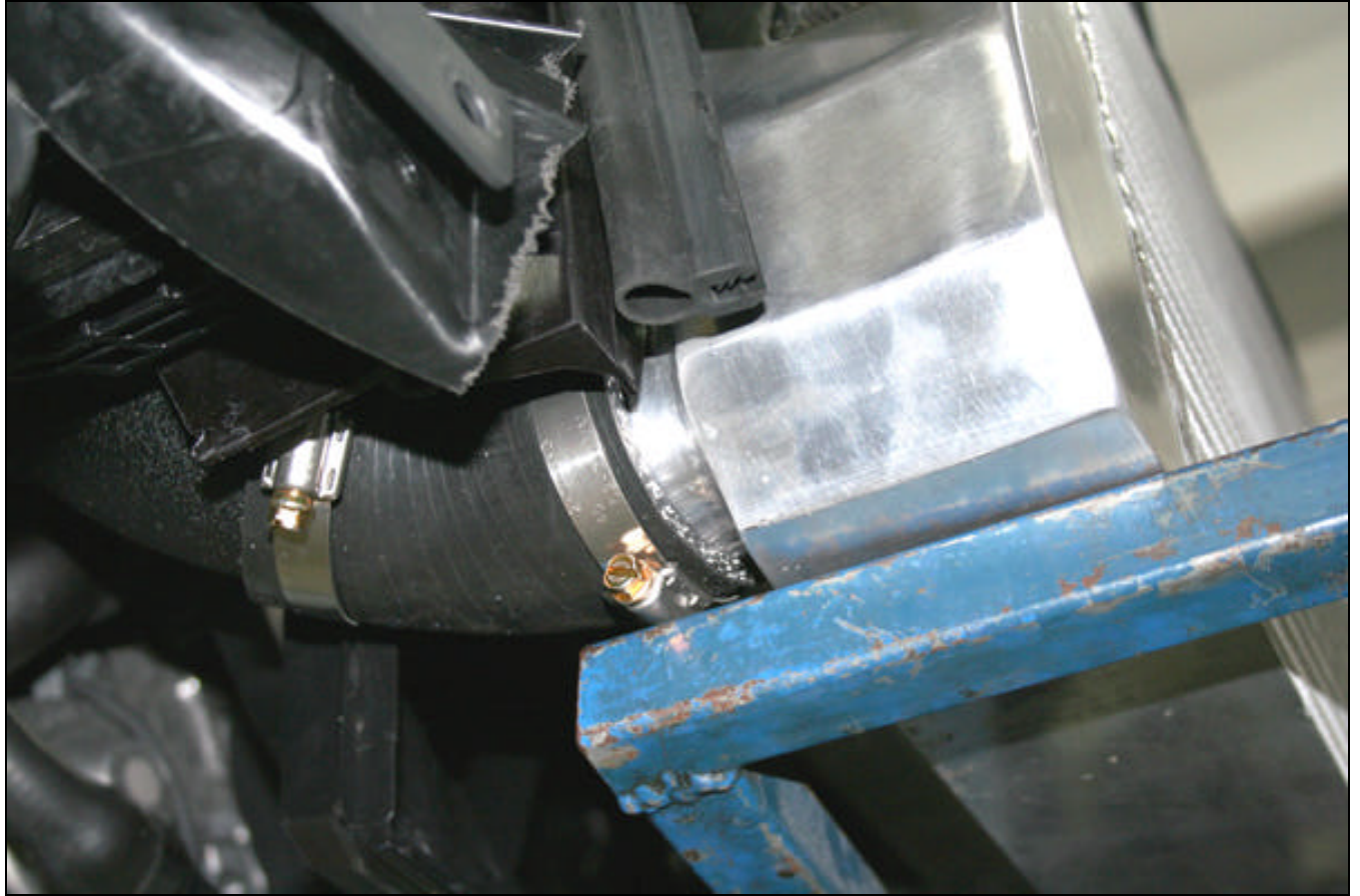
Passenger side hose and pipe installed to intercooler
