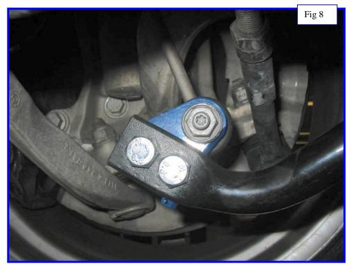
9. Bolt the drop link in hole #1 and torque to factory specs. Repeat for other side. (See Figure #8)
