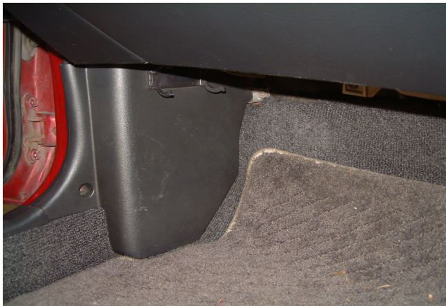
Figure 7 – Kick panel Re-installed
