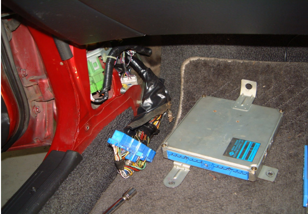
Figure 2 – Factory ECU disconnected and removed
