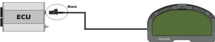
Figure 9 – Haltech ECU connected to a Racepak Dash
