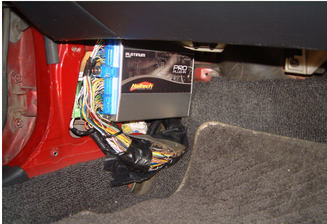
Figure 6 – Platinum Pro Plugin Mounted in a R32 GTR.
