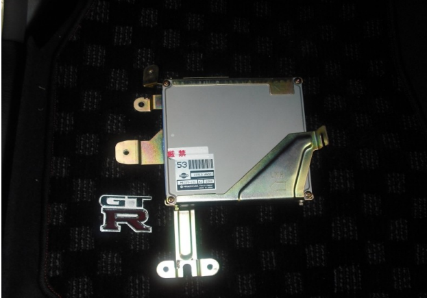
Figure 2 – Factory ECU disconnected and removed
