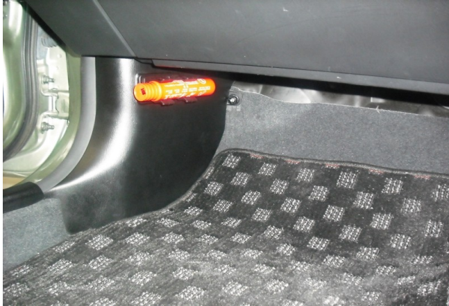
Figure 6 – Kick panel Re-installed
