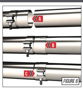
Install each exhaust tip with the included T-bolt clamps, but do not torque until the exhaust system has been fully adjusted and tip placement is satisfactory.
