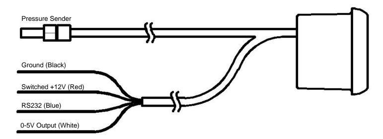
Figure 1. Connection Diagram
