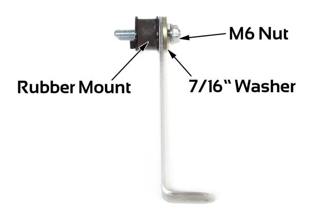
9. Install supplied bracket (with rubber mount) to threaded hole in frame rail and secure using supplied M6 bolt and fender washer. Leave loose until air intake pipe is mounted.
