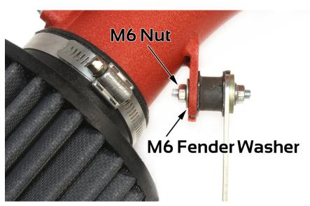
16. Adjust intake tube so filter and other parts are at least 3/8" away from chassis and other immovable objects.
