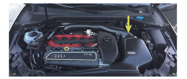
► Locate the solenoid valve as indicated
