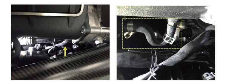
Disconnect the original vacuum tube and install a T-connector to create a vaccum source
