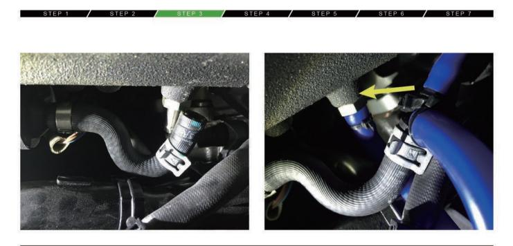
Disconnect the original vacuum tube and install a T-connector to create a vaccum source
