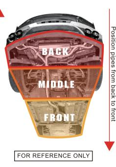
Tighten pipes from front to back
