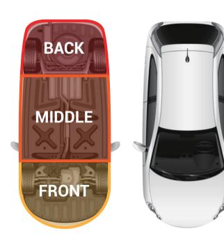
Tighten pipes from front to back
