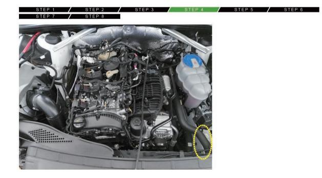
Locate the solenoid valve as indicated
