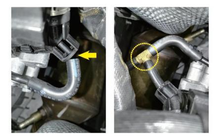
Disconnect the original vacuum tube and install a T-connector to create a vaccum source
