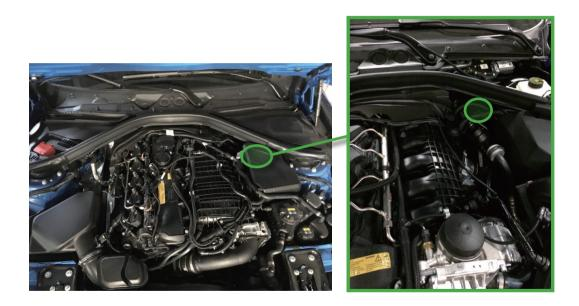
► Locate the solenoid valve at the indicated location
