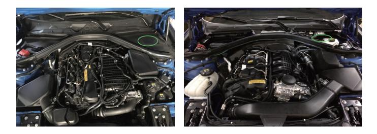
▶ The vacuum source is located at the top right quadrant of the engine bay
