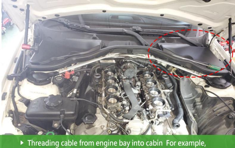
► Threading cable from engine bay into cabin For example, threading iron wire from cabin into engine bay and drag cable into cabin
