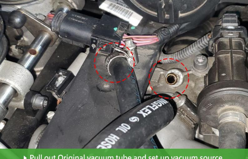
▶ Pull out Original vacuum tube and set up vacuum source
