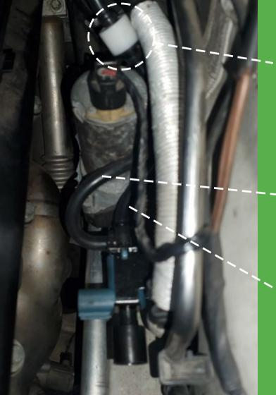
The white end of one-way valve should point to vacuum source
