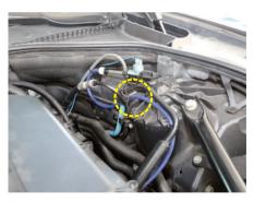
▶ Install the vacuum tube to the solenoid as shown.
