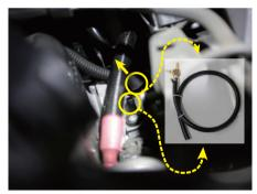
► Connect the vacuum tube as shown.
