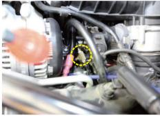
▶ Install the T-connector and connect the vacuum tube then return it the original position.
