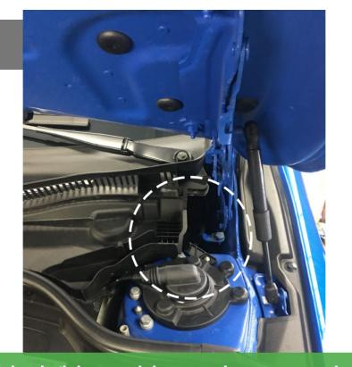
► The black/blue cable needs to pass through the area indicated from the engine bay to the cabin. #Note that you need to make an incision on the rubber block to make way for the cable to pass through. Seal it with an adhesive to prevent water damage.
