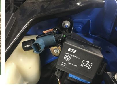
▶ Install the solenoid valve here
