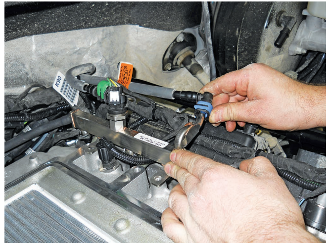
9. Locate 1320-15799SLV-AB found in 1121-HWKB, install over fuel line to prevent chaffing.
