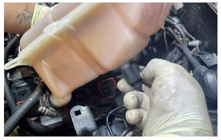
**Step 19** Swing the coolant reservoir out of the way.
