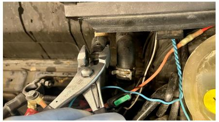
**Step 11** Using an 8mm socket, loosen the hose clamps on the y-pipe.
