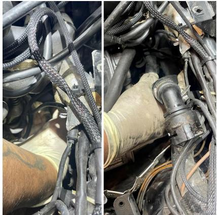
Step 21 Push down on the grommet containing both hoses to separate it from the firewall.
