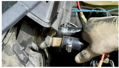
**Step 28** Use the grommet to seal the opening.
