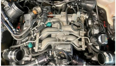
**Step 15** Using a small pick, release the clip from the passenger side heater core hose connector. It's down between the motor and the firewall.
