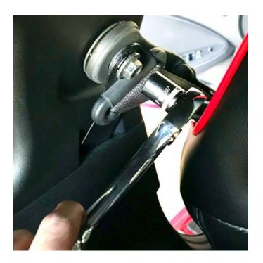
Step 3: Use OEM top seat belt mount bolt and spacer (14mm) and tighten the harness bar in on both sides. (There should be an additional spacer that BRAUM provides if you do not plan to use your OEM seat belt)
