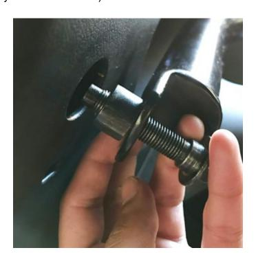
Step 4: Secure the top of the support arms to the harness bar using Allen Key (6mm).
