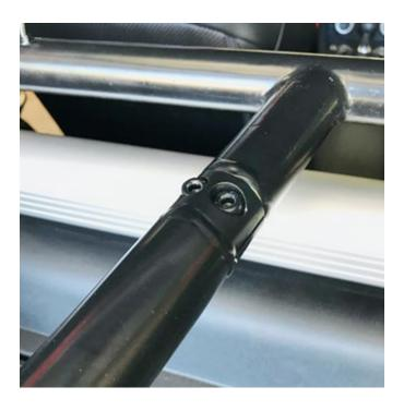
Step 5: Secure the bottom of the support arms to the chassis points in the spare tire compartment using the 13mm socket wrench.
