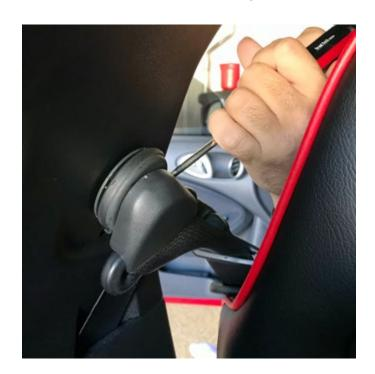
Step 2: Use 14mm socket wrench to take off seat belt top mounts on both sides.
