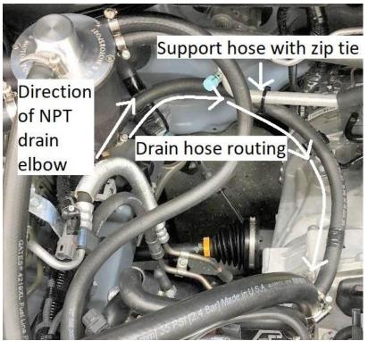
NOTE-This fitting is tapered- do not force the fitting to thread in beyond 60% of the fitting's thread length. The fitting should thread in approximately 3 revolutions before you need to use a wrench. Expect to see approximately 3-4 threads remaining once installed. The AOS may not drain effectively if the fitting is installed too deep/too tightly.
