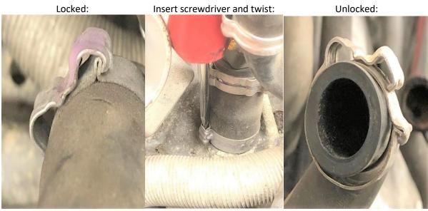
Remove one ½" clamp and hose from the smallest of the two rocket cover ports: \*\*\*NOTE: 2002-2005 WRX: there is only one hose and port on each rocker cover. The driver side rocker hose goes to a short hard pipe. The passenger side hose goes to the black PCV pipe (mounted to the intercooler)
