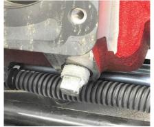
To remove the pcv assembly from the vehicle, locate the OEM ¾" diameter hose that the pcv connector is installed in. Loosen the clamp closest to the block (the clamp closest to the engine block, furthest down) by using a narrow flathead screwdriver: insert it into the gap in the side of the clamp and twist. With the clamp unlocked, twist the hose and pull up on the ¾" hose to remove it. Set aside for storage.
