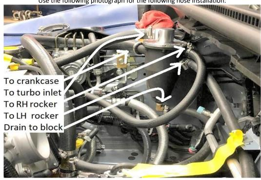
Take the unused end of the ½"x32" drain hose (the hose that intersects perpendicularly into the tee) and install it on the AOS drain fitting with a clamp. The hose should appear to route in a U-shape. You may secure it to an AC line with a zip tie, this will help prevent the hose from sagging and contacting the downpipe.
