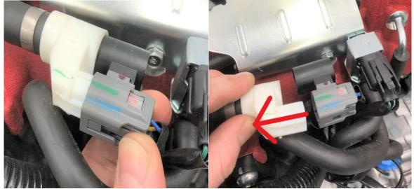
With needle nose pliers: pull metal shorting bar straight back while holding white connector:
