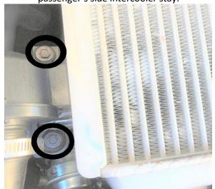
Remove the 12mm bolt that secures the intercooler to the passenger side intercooler stay(bracket).
