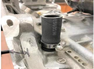
Once the hose is installed on the block and secured, insert the tee into the  $\frac{3}{2}$ "x2.5" hose and secure it with a clamp. Be sure to position the  $\frac{1}{2}x32^{2}$  drain hose so that it points back toward the firewall. This hose will soon be routed to the bottom of the AOS.
