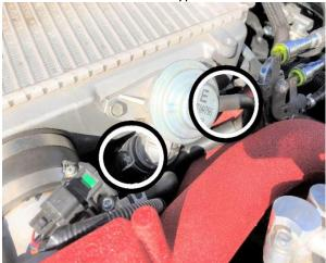
(Removing the intercooler from the vehicle with bypass valve attached prevents you from having to replace the single-use bypass valve gasket.
