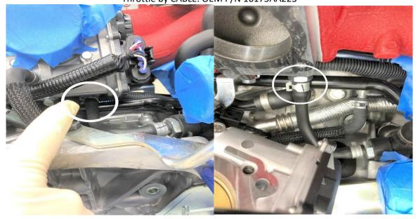
Using a 19mm deep well socket, remove the barbed fitting from the intake manifold. Set Aside for
