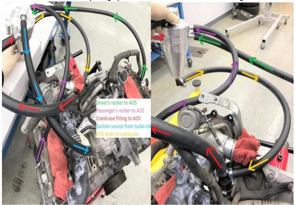
Double check all clamps, hardware and fittings for secure fitment. Reinstall the intercooler, secure related clamps and brackets.
