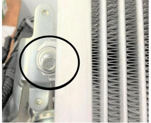
Remove recirculation hose from bypass valve by compressing the hose clamp with pliers until they lock in the open position. Push the recirculation hose off the bypass valve fitting. Disconnect boost/vacuum hose from the bypass valve.
