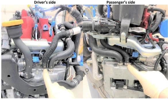
Perform this once on each rocker cover. Use a narrow flathead screwdriver to release the locking clamps: insert screwdriver in the gap on the side of the clamp, twist screwdriver to disengage clamps. Remove one ½" hose from each rocker cover port. Leave these hoses attached to the black breather pipe, which was fastened to the intercooler- leave it in place for future removal.
