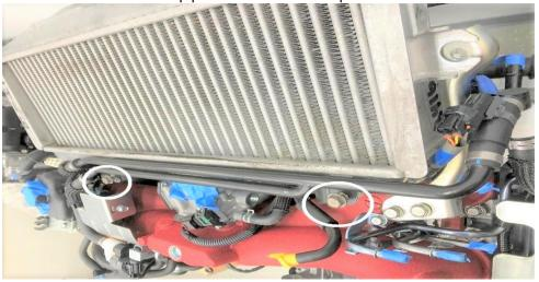
Remove intercooler from vehicle and set on a workbench, in a clean area. Apply tape over inlet and outlet. Wipe oil (with microfiber) from throttle body, intake manifold and intercooler if found)
