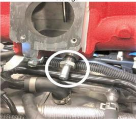
Install the supplied NPT plug in the intake manifold with teflon tape or thread sealer. Expect to see 4-5 threads remaining once the plug is installed correctly.
