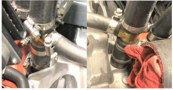
Install one end of the 5/8"x24" hose on the fitting on the front of the turbocharger inlet, with a clamp. White connector is removed, clip transferred to engine harness grey connector and sealed off.
