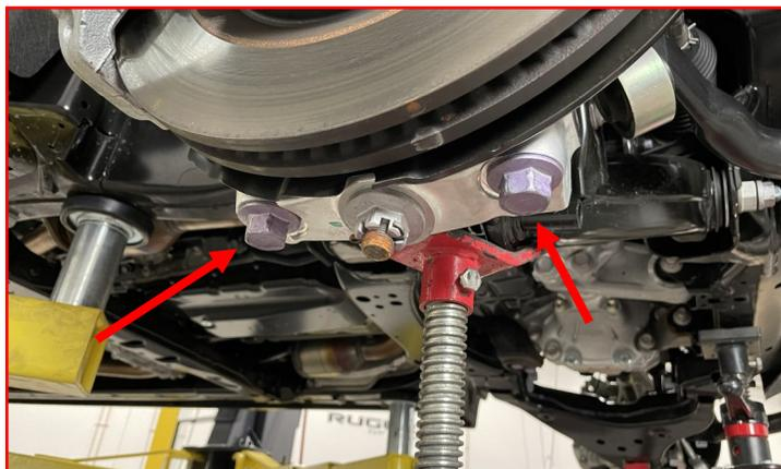
Torque the upper strut **hardware** to **40 ft-lbs**.
