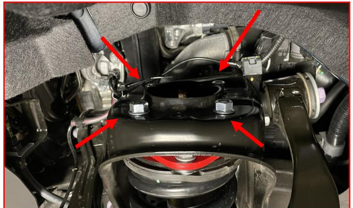
Using **factory hardware**, rise the lower control arm enough to install the lower strut bolt.
