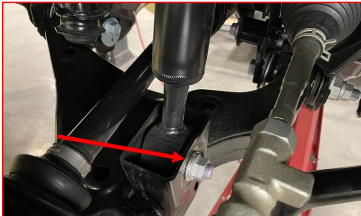
Remove the four (4) **upper strut bolts**.
