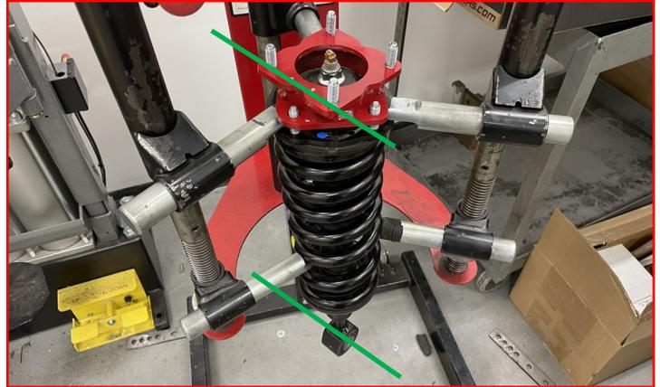
Carefully remove the strut from the spring compressor.
