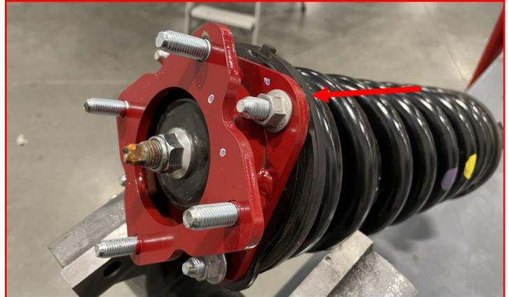
Insert the strut and spacer assembly into the vehicle and install using the **supplied M10x1.25 serrated flange nuts**.
