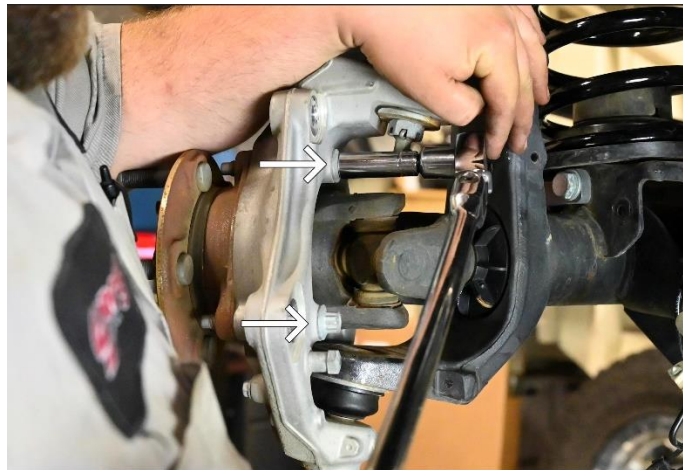
Figure 22. Unit Bearing/Hub Bolt Install
