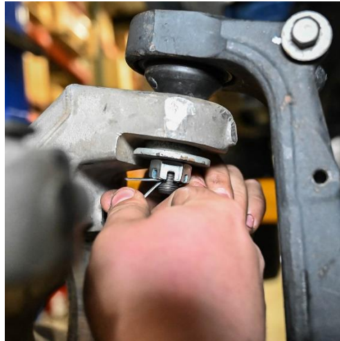
Figure 21. Properly Aligned and Installed Cotter Pins
