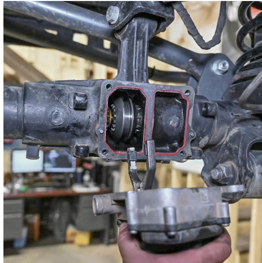
Figure 23. Front Axle Disconnect Motor Reinstallation
