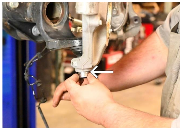
Figure 18. Reinstalled Knuckle with Lower Ball Joint Castle Nut Lightly Tightened
