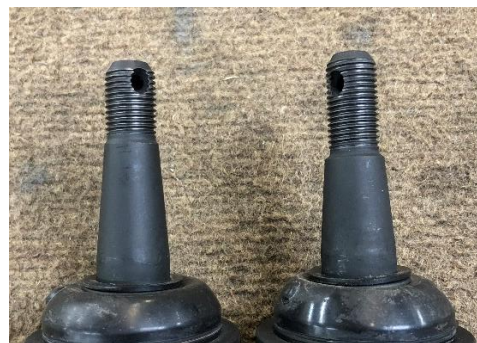
Figure 15, Difference in Threaded Stud Lengths. (Left – Lower, Right – Upper)
