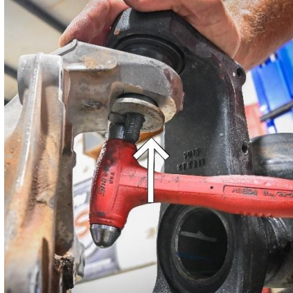
Figure 19. Proper Tapered Bushing Install with Hammer
