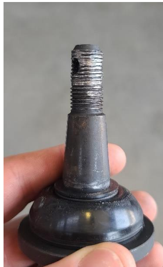
Figure 20. Damage Resulting from Improper Installation of Tapered Bushing
