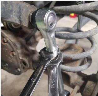
Figure 4. Tightening the tie rod end jam nut.
