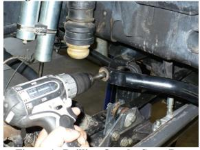
Figure 1. Drilling Out the Sway Bar
