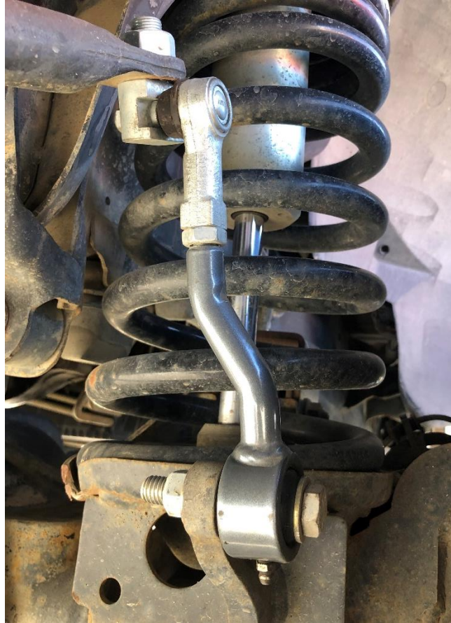
Figure 4. Correctly Installed Sway Bar End Link (2003-2013)
