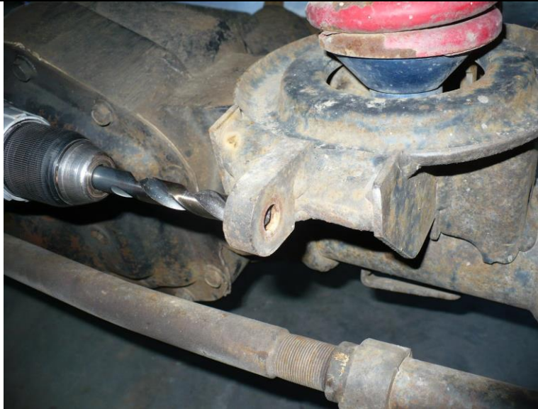
Figure 2. Drilling Out Lower Mount to 1/2"
