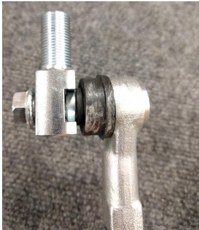
Figure 3. Properly Assembled Sway Bar End Link
