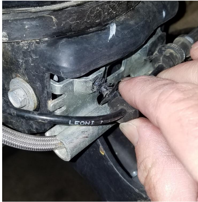
Figure 9. Reinstalling ABS Wiring Mounts.
