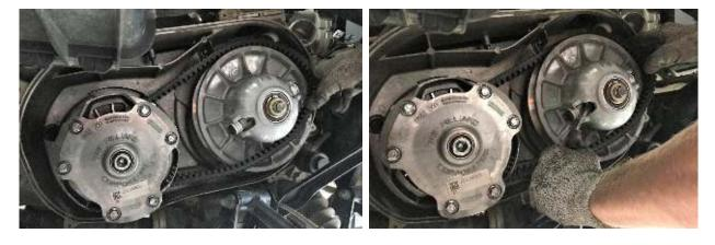
12. Install NEW outer clutch cover housing provided with kit. Ensure seal is good or replace.
