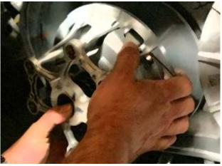
3. Pull the Polaris primary fixed sheave from the engine crankshaft using PN 99-012 puller. Greasing the end of the puller slightly will aid in removal. Do not get grease on any clutch components.
