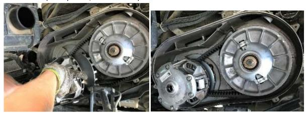
7. Install DURACLUTCH Primary with shoulder washer as shown. <u>DO NOT USE</u> the O.E. flat washer or lock washer. The flat washer will interfere with the primary cover. Tighten bolt to **60 ft-lbs**. **VERY IMPORTANT-** Over tightening will not allow clutch to operate properly and cause damage and failure of the clutch.
