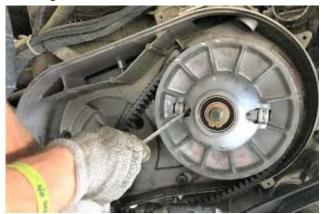
7. Slide belt into primary clutch, then install on post.
