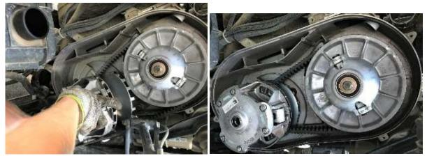
Install DURACLUTCH Primary with shoulder washer as shown. <u>DO NOT USE</u> the O.E. flat washer or lock washer. The flat washer will interfere with the primary cover. Tighten bolt to **60 ft-lbs**. **VERY IMPORTANT**- <u>Over tightening will not allow clutch to operate properly and cause damage and</u> <u>failure of the clutch</u>.
