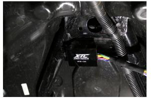
3. Take the short Harness KAV-SV3, starting at the driver side, un-plug the taillight and plug the harness with the yellow wire inline, run the other connector to the other side and plug it inline with the right taillight.
