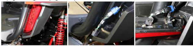
WARNING! Keep power wire away from any hot or moving parts.
