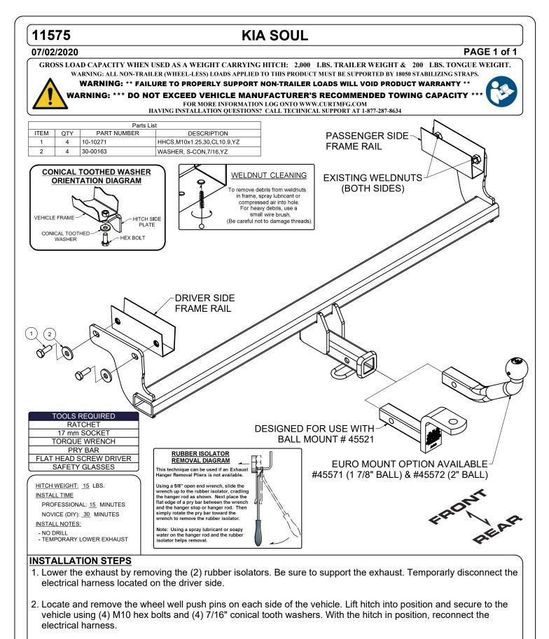
3. Torque 10mm hardware to 48 ft-lbs. Raise exhaust back into position and secure to vehicle hangers. Reinstall push pins removed in step 1.
