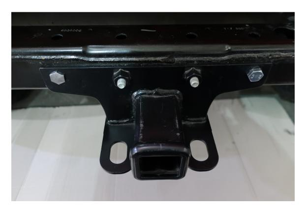
6. Replace right side (passenger) bolt with 12mm x 1.75 x 100mm. Head of bolt to rear of Jeep using 18mm wrench.
