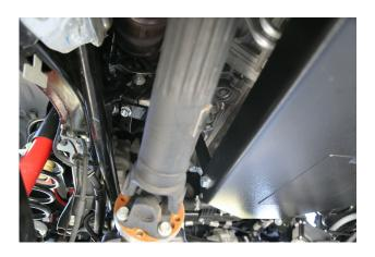
9. Install oil pan skid plate right/passenger side drop bracket in rear hole under motor mount hole using 1x ½" x ¼" hex bolt with ½" washer and ½" nylock nut.
