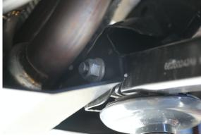
13. Tighten all skid plate hardware at this time.
