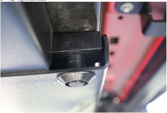
6. Install 3 fuel tank brackets into nuts in undercarriage with 3x 12mm x 1.5 x 35mm bolts. Hang fuel skid to brackets with 3x 3/8 x 1 hex bolts and 3x 3/8 nylock nuts. Remove 2x frame side factory bolts. Slip front of skid between cross member and belly pan skid.
