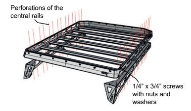
Tighten all the screws to finish with the installation.
