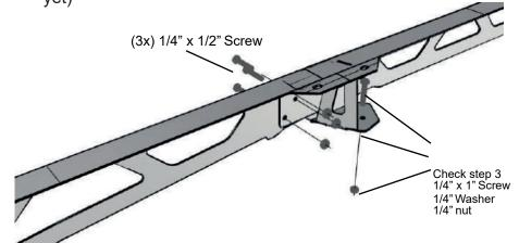
Settle the leg over the roof (only with the original roof), place a washer over the perforations as it shown in the image, using 1/4" x 1" screws. (Do not tighten yet)
