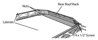
Place the frontal corner with the lateral (as it is shown in the image). Use four 1/4 x 1/2" screws with nut (Do not tighten yet).
