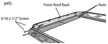
Align 4 central bars with the perforations (as it is shown in the image). Use twelve  $3/16 \times 1/2$ " screws with nut, inserting them bottom-up and tighten all screws.
