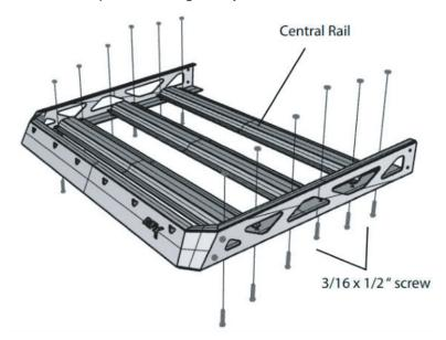
Place the rear rack with the front rack, aligning Bracket with the perforations (as it is shown in the image), using eight 1/4 x 1/2" screws with nut. (Do not tighten yet).
