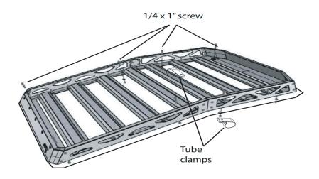
\* For safety tighten all the screws. Now you have completed the installation.
