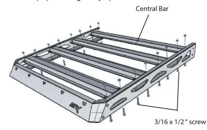
Place the rear rack with the front rack, aligning the "C" hardware with the perforations (as it is shown in the image), using eight 1/4 x 1/2" screws with nut. (Do not tighten yet).
