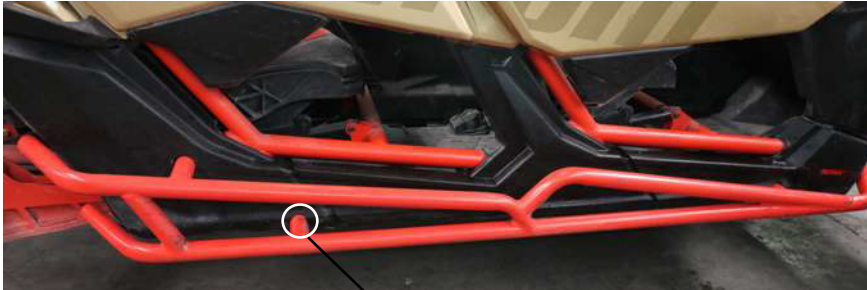
Central Tube with 3/8 x 2 1/2" screw.
