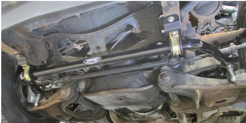
Figure 11 - Installed Sway Bar
