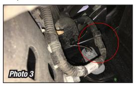
Unplug the factory fog light wiring harness from the vehicle side harness on the inside of the drivers side frame rail, behind the bumper. Shown in photo 4.
