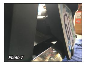
10. With the plastic filler removed from the center, you can now trim the remaining plastic pieces on the inside of the tow hook area. The plastic is easily cut with a sharp razor knife. Trim along the line shown in silver, and pointed out by the arrows first to retain rigidity to the plastic surround. See photo 8. You can loosely attach the KD Fabworks brackets to your light bar and test fit to see how much you need to trim.
