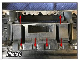
9. With the center bolts and push in retainiers removed you can pull out the center section of the plastic filler, with the license plate attached. You will have to pry up a bit on the license plate to get it to slip over the lower bumper lip as you pull the assembly out the back of the bumper.
