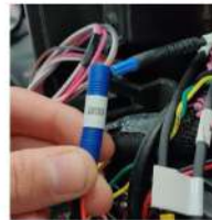
Camera Harness (Plugged into 360 ECU)
