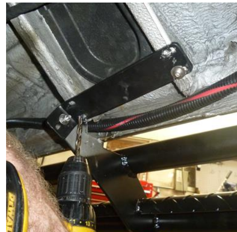
Figure 6. Center mounting bracket against front body brace.
