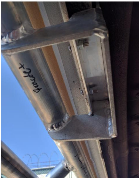
Figure 4a and 4b. (below and bottom right) Front mounting brackets against pinch weld of van.
