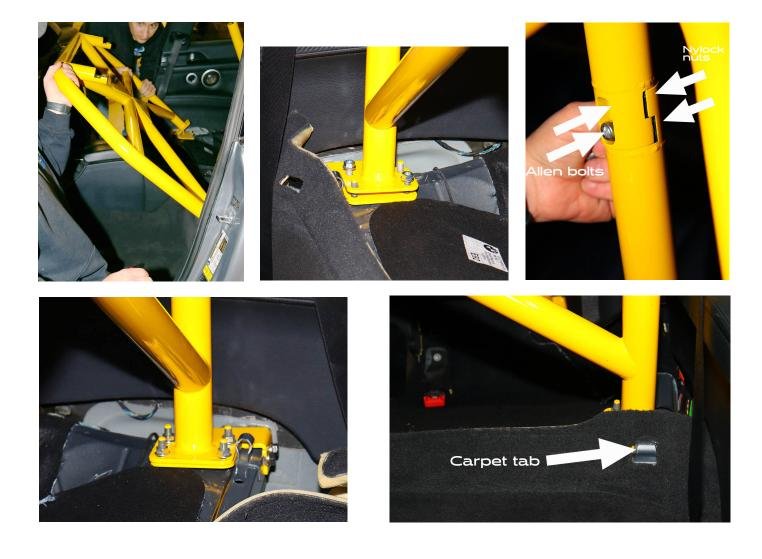
Replace the carpets using the metal carpet tabs, reinstall your seat if necessary, and you're done. Don't forget to reconnect the battery!
