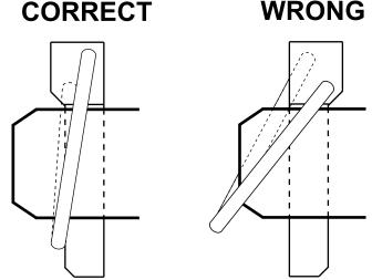
IMPORTANT: When properly installed, the ring on the Click Pin will "snap" against the shaft of pin. When installed backwards, the ring does not fit snugly against shaft.
