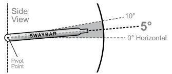
IMPORTANT: DO NOT exceed Maximum Length (measured from center-to-center of bushings) indicated for your part number.
