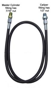
The extra 7/16-24 fitting is so the brake line will fit the IQ chassis. Replace the Master Cylinder fitting (7/16" nut) with the extra fitting (1/2" nut).
