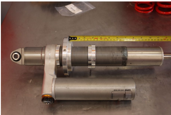
Set the crossover ring to 85mm from the spring seat to the bottom of the crossover ring.
