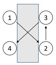
Tighten u bolts in a cross pattern a little bit at a time until each nut is torqued to 100 ft-lbs.
