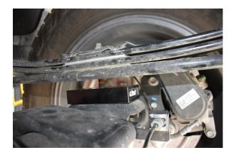
Insert the lift block with the pin pointing down located in the hole on the axle pad
