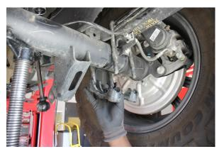
Remove the U bolts and bracket securing the axle to the leaf spring
