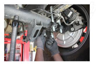
Install the OE axle carrier and the provided washers and nuts and hand tighten so each end is evenly tightened. Do not tighten completely at this point.
