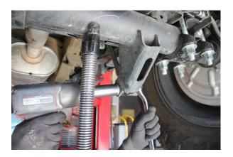
Reinstall the lower shock mount to the shock
