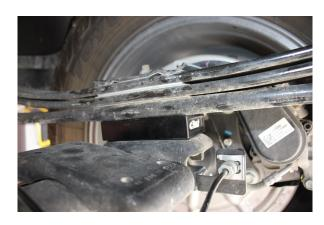
Raise the axle so the locating pin on the bottom of the leaf springs is located in the hole on the top of the lift block
